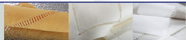
"Jour de Venise" is obtained by using in first operation Cornely 15 thread pulling machine and in second operation Cornely 10-X double needle ladder stitching machine.
